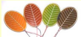
Leaf-shaped transparent DSC with four colors
