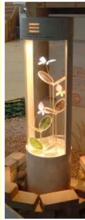
Leaf-shaped transparent DSC with four colors
