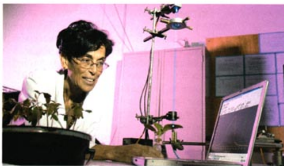
Pollution patrol. The author uses laser-induced fluorescence analysis to detect pollutants in plant tissue.
