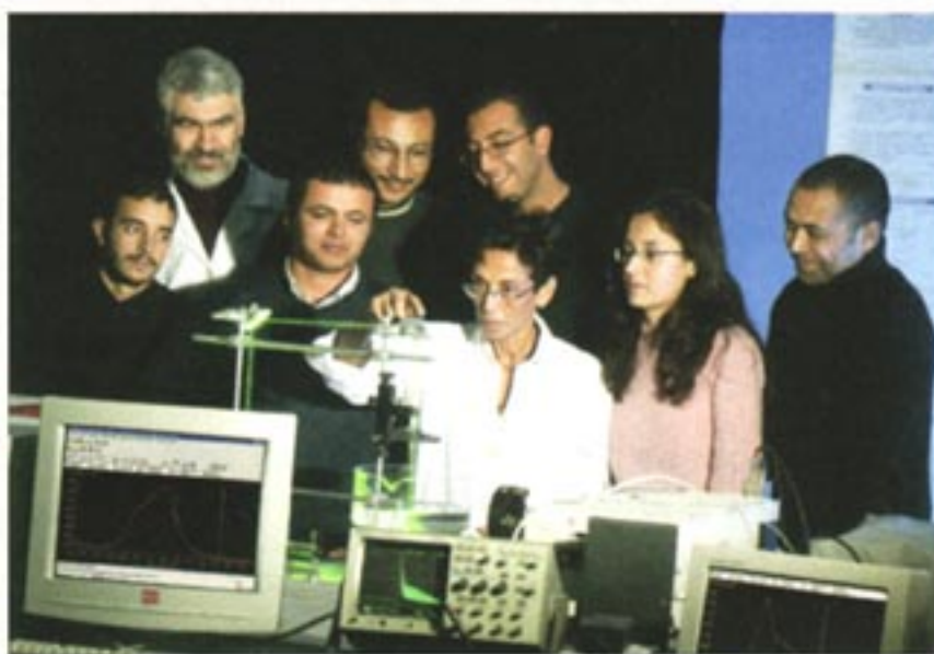
Science huddle. Surrounded by colleagues, Zohra Ben Lakhdar analyzes water for pollutants using a technique called laser-induced breakdown spectroscopy.
